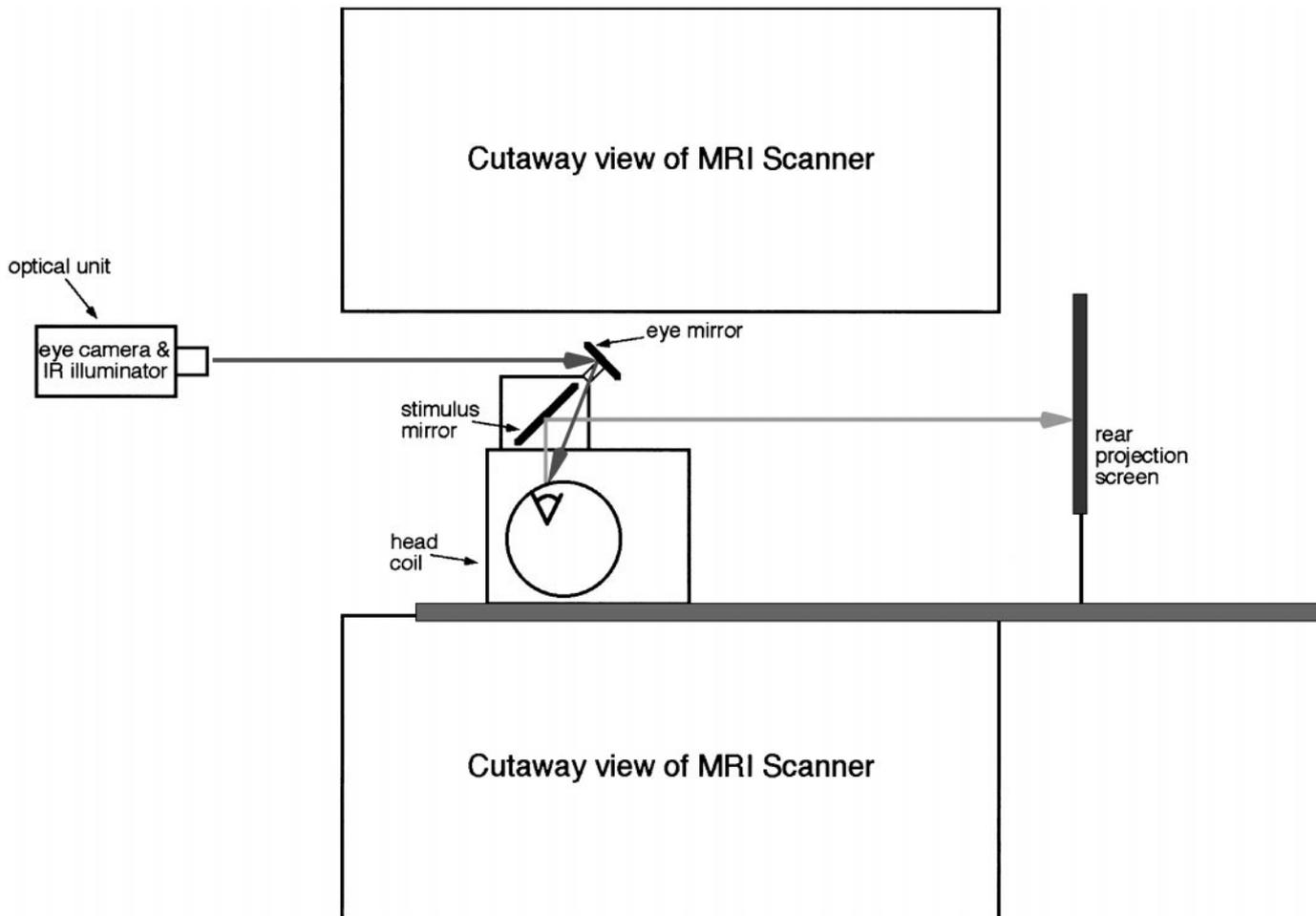
**FIG. 1.** Schematic of the mirror system on the head coil illustrating the light paths for both the optical unit and the subject. The positions of the mirrors allow unobstructed views for both the eye camera and the subject. During imaging, the subject can see only a minimal dull red glow of the infrared light source if he or she looks directly into the eye mirror.
